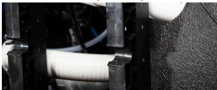
French Cleat (top) and C-Clip (bottom)
