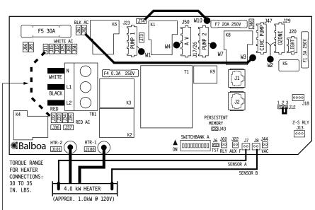
CONNECT ONLY TO CIRCUITS PROTECTED BY A CLASS A GFCI.
