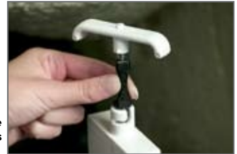
Step 2 : Check Slice Valve Keepers
