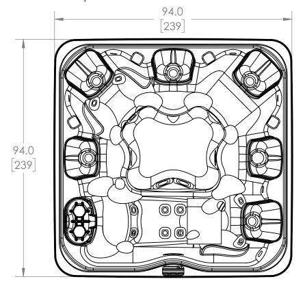
89.6 228 FROM BOTTOM 28.7 OF BASE 73 89.6 228 FROM BOTTOM OF BASE 35.0 35.0 89 89 5.0 \* Ø 3.0\* EURO RATINGS/WIRING CONFIGURATIONS AVAILABLE: [13] 230 VAC, 50 Hz, 16A x 1 230 VAC, 50 Hz, 16A x 2
