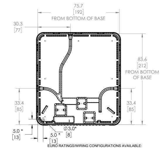
230 VAC, 50 Hz, 16A x 1 230 VAC, 50 Hz, 16A x 2 230 VAC, 50 Hz, 32 A 400 VAC, 50 Hz, 16 A x 3 (3 phase)
